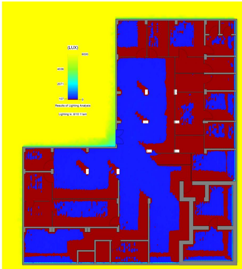
Figure 19 Light Analysis Results Study of Al-Rafidain Bank building in Al-Mansour
