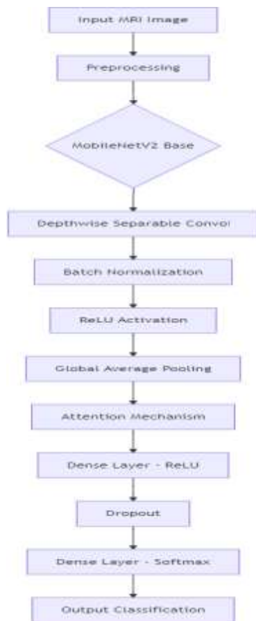
Fig. 2: Detailed configuration of MobileNetV2 layers within the model.
