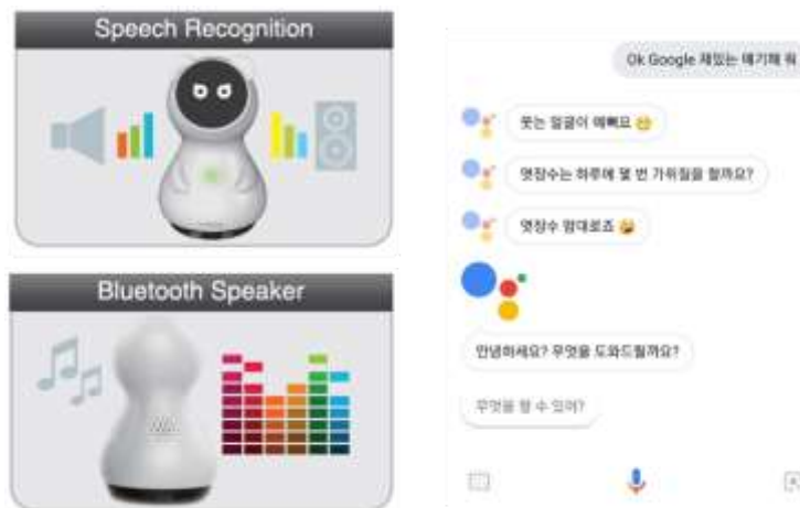
Fig. 2. Bluetooth Microphone and Speaker for Speech Recognition and TTS Functionality of the Bingle-S Robot, Enabling Advanced Voice Interaction for Educational and Entertainment Purposes
