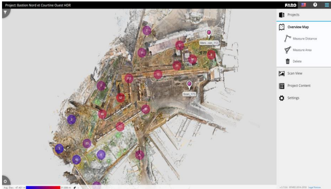
Figure 7. WebShare viewer of the North-West Bastion, used for verification and measurement.
